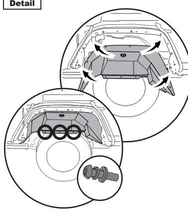
Having Followed the Fender Liner instruction sheet, Double check and make sure to connect rocklight wiring (optional), and be sure that the Liner flange is inside the body side fender lip in all locations.
