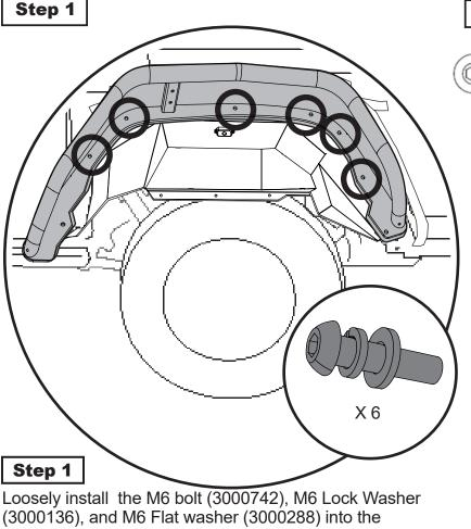
Loosely install the M6 bolt (3000742), M6 Lock Washer (3000136), and M6 Flat washer (3000288) into the Bestop Aluminum Wheel Liners (4966501). Install directly into the Rivetnut that are on that assembly.
