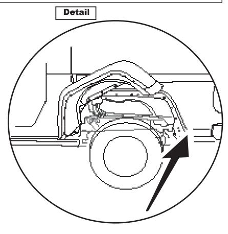
With the inner liner fasteners removed and loose, now you can remove the entire fender. Grab the fender and pull the fender away from the body. It's attached with clips.
