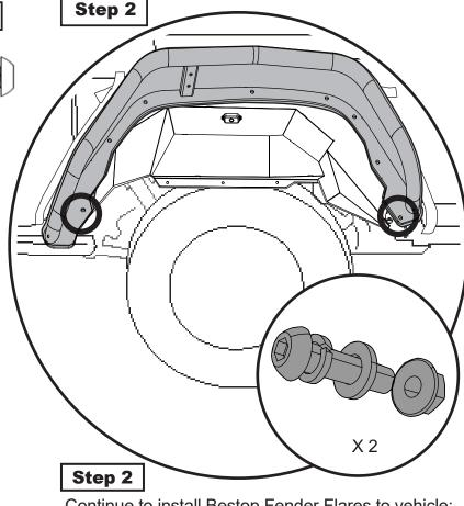
Continue to install Bestop Fender Flares to vehicle: Loosely install the M6 bolt (3000742), M6 Lock Washer (3000136), and M6 Flat washer (3000288), in the locations that do not go into the fender liners, and are accessible to the back side.
