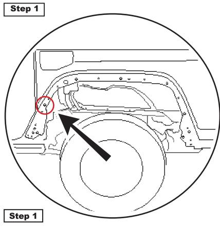
In order to proceed, make sure that all the One (1) hole (shown red) on each forward (cab side) of the truck wheelwell are drilled. Use the 10mm (25/64") drill to open up these holes for the nutserts, and the holes are properly treated for metal protection
